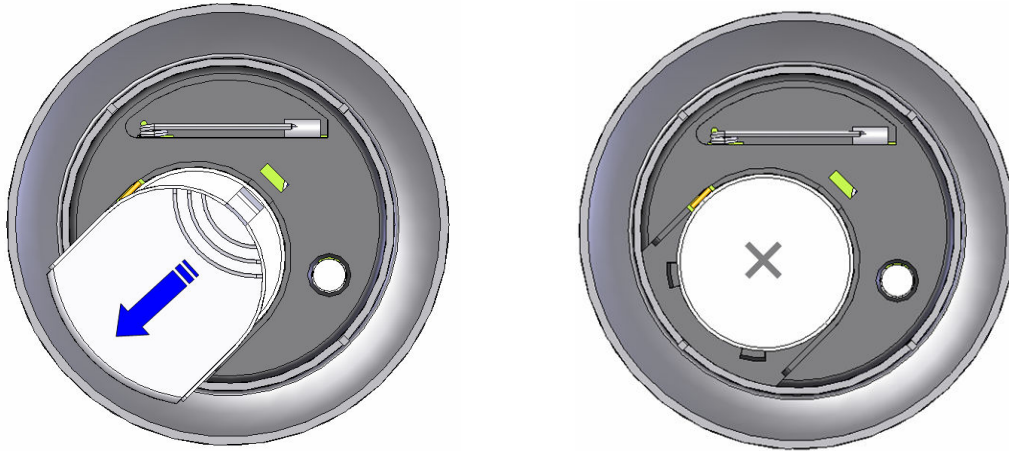
Figure 3 removing battery cover of the Tag and inserting the battery.
